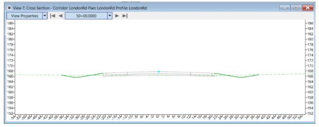
Note that **Dynamic Cross Sections** are displayed in specially defined cross section model views. Any view can be defined to display the dynamic cross sections.
