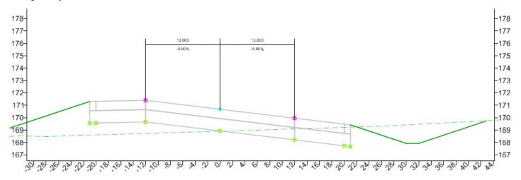
9. Navigate through the cross sections and notice how the slopes change based on the superelevation that has been applied.
