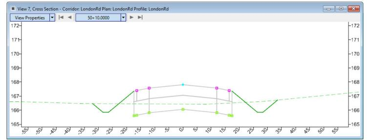
Note, the magenta boxes that appear at the left and right edge of pavement point locations on the cross sections. These boxes indicate a superelevation point control has been created and assigned to the corridor.
